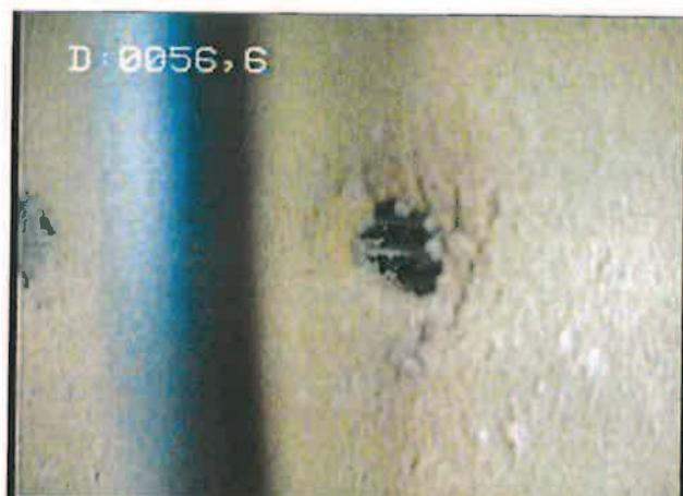
**Tube plein de 56,6m à 60,2m.****Niveau de filtre inférieur entre 60,2m et 60,7m.**
